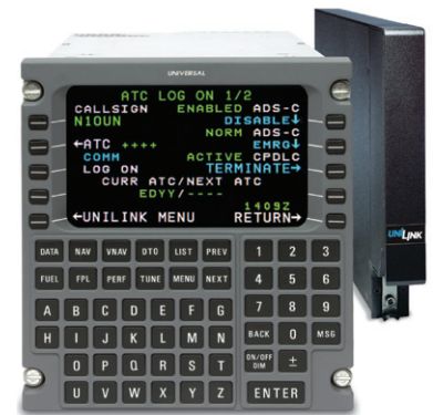
UniLink UL-800/801 Communications Management Unit (CMU) Airborne Datalink System
