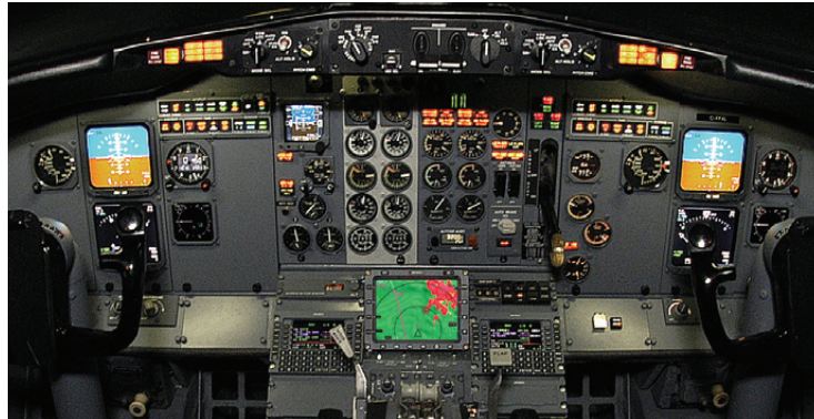
MC2 Mods to Air Inuit B737-200C featuring Universal Avionics WAAS/SBAS-FMS, TAWS and MFD-640. Photo credit – MC2.
