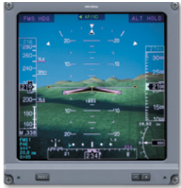
SVS Egocentric View displayed on an EFI-890R Primary Flight Display
