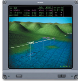
SVS Exocentric View displayed on an EFI-890R Navigation Display
